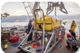
The success of the first sea trials of the Ulyx underwater drone, the new technological jewel of **the French oceanographic fleet** operated by Ifremer. Ulyx is the first drone capable of carrying out a 24-to-48-hour mission at a depth of 6,000 meters in complete autonomy. It will be operational for its first scientific missions in 2022 ([link to the video](#)).
