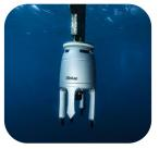
Remotely Operated Vehicle R7 and GAPS acoustic system
