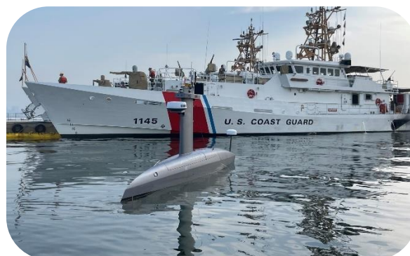
DriX unmanned surface vehicle
