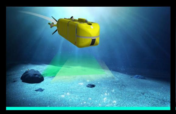
**Ulyx**, a deep sea autonomous drone delivered to IFREMER, able to operated at 6,000 m depth for 48h
