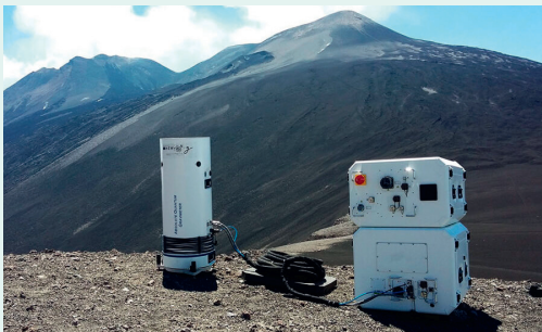
Quantum gravimeter deployed on Etna, in Sicily
