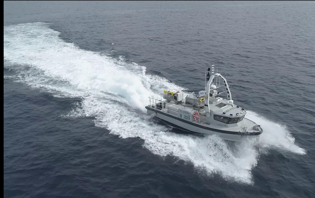
Autonomous surface vehicule carrying underwater drones to survey area (USV)
